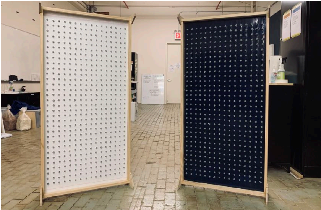
Fig 17. Two LED Screens, Framed and Ready for Action
